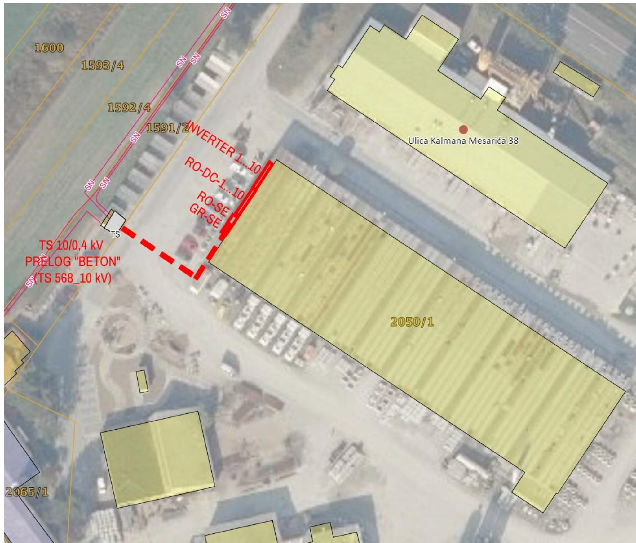
Prilog 6: Prostorni raspored opreme FN elektrane
